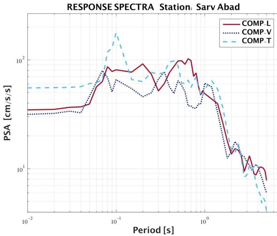
Figure 14. Acceleration response spectra at Sarv Abad station at about 68 km epicentral distance.
