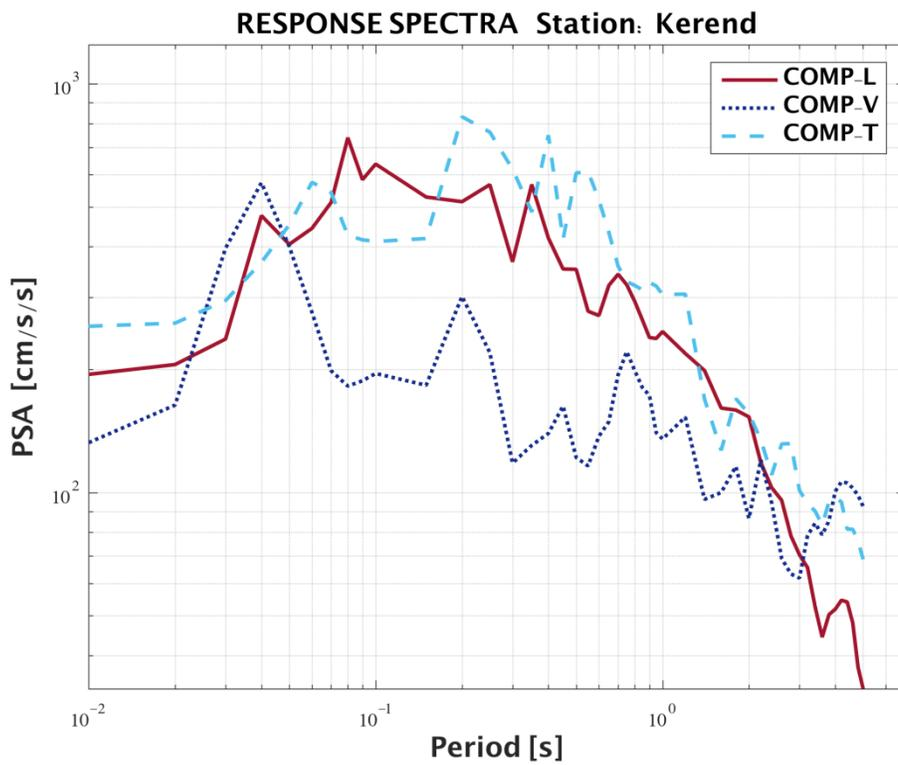
Figure 10. Acceleration response spectra at Kerend station at about 70 km epicentral distance.
