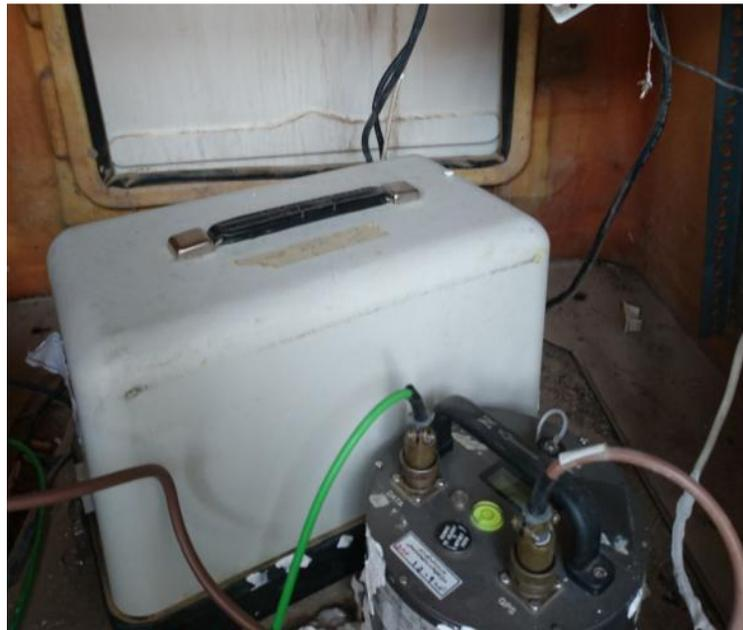
Figure 3. Sarapol-e Zahab station (SSA-2 permanent instrument along with the temporary CMG5TD instrument).
