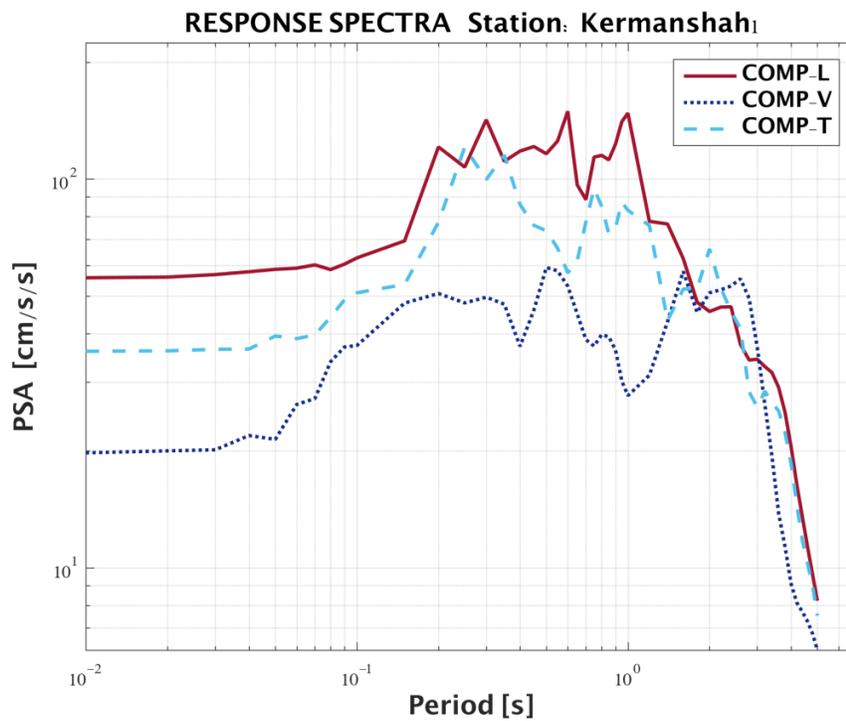
Figure 24. Acceleration response spectra at Kermanshah1 station at about 122 km epicentral distance.
