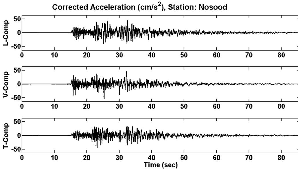
Figure 11. Recorded acceleration time history at Nosood station at about 45 km epicentral distance.
