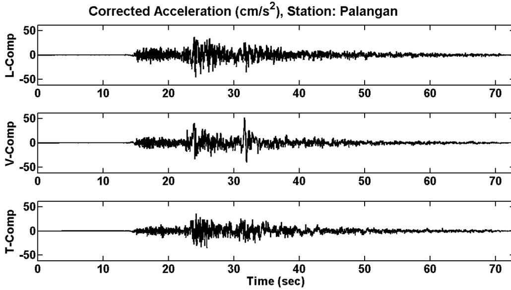
Figure 15. Recorded acceleration time history at Palangan station at about 69 km epicentral distance.
