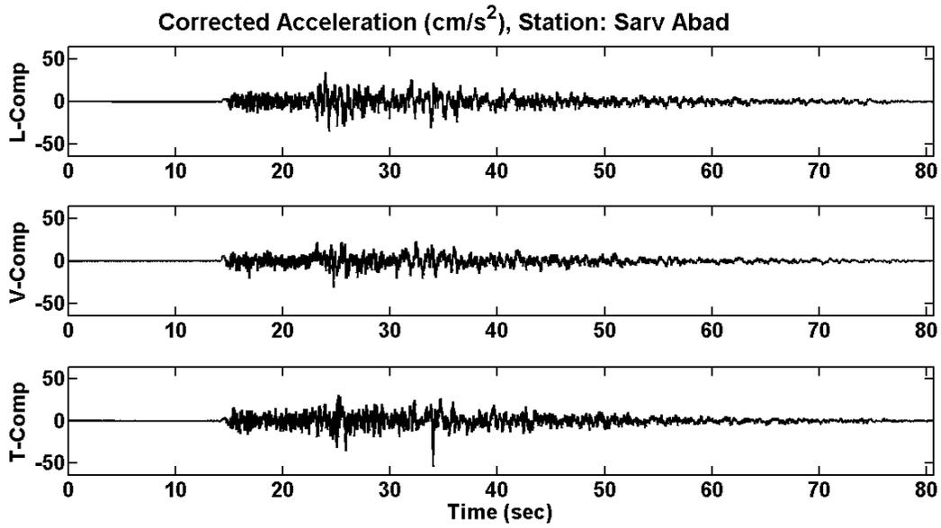
Figure 13. Recorded acceleration time history at Sarv Abad station at about 68 km epicentral distance.
