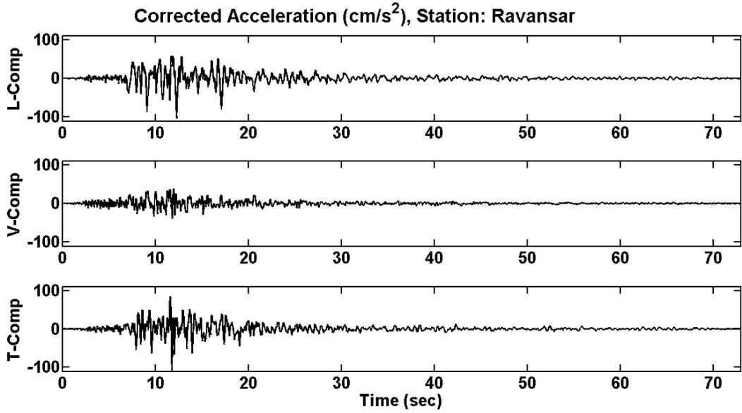
Figure 17. Recorded acceleration time history at Ravansar station at about 72 km epicentral distance.
