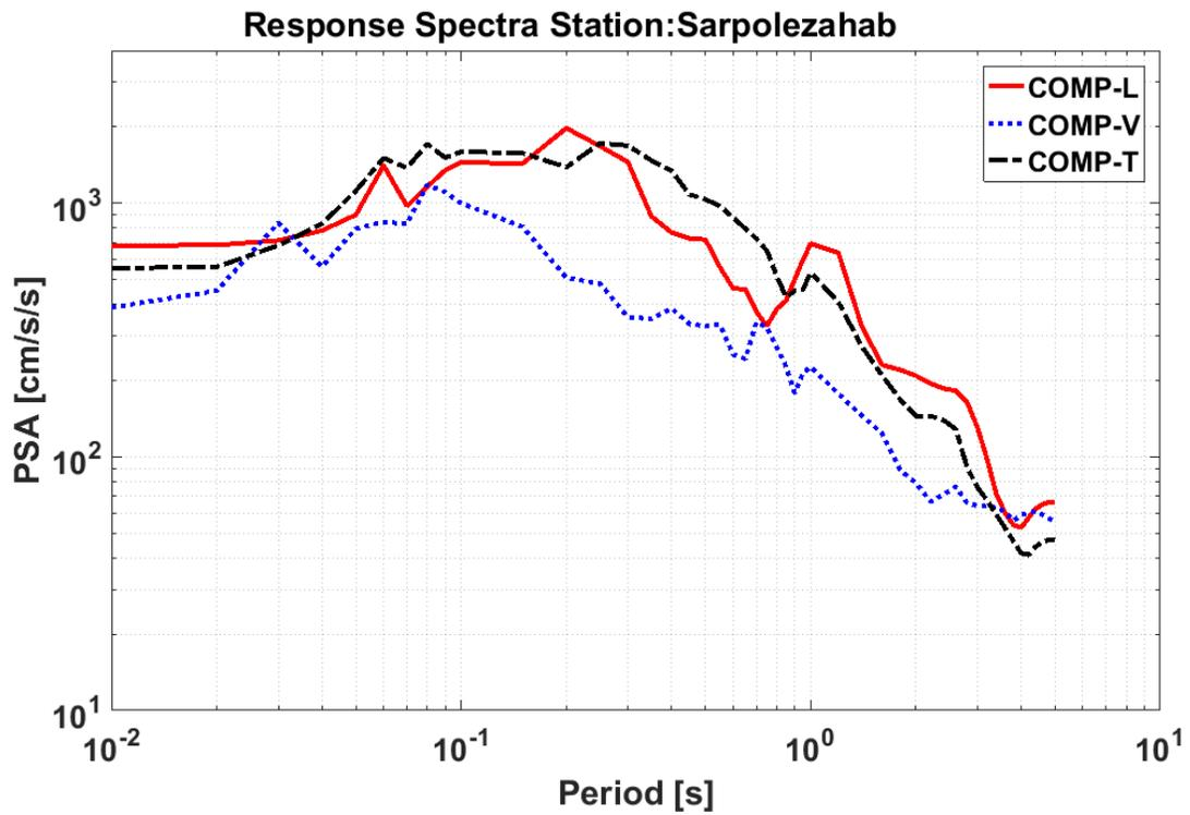
Figure 5. Acceleration response spectra at Sarapolezahab station at about 40 km epicentral distance.
