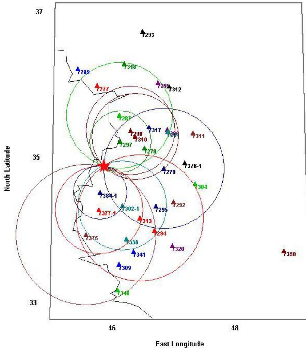
Figure 8. Epicenter location determination using the recorded accelerograms.
