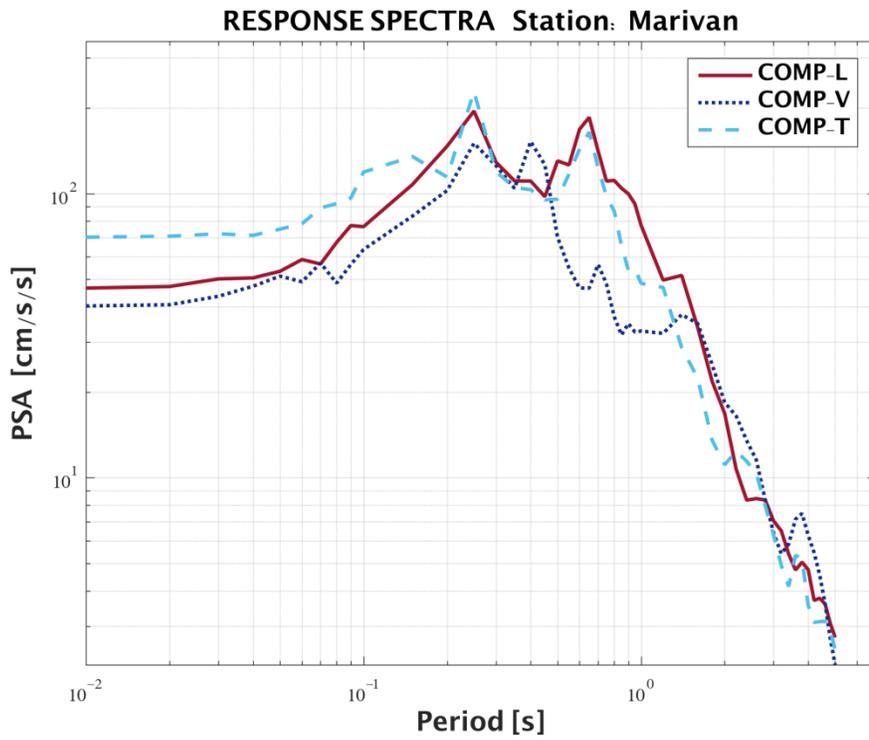
Figure 20. Acceleration response spectra at Marivan station at about 80 km epicentral distance.
