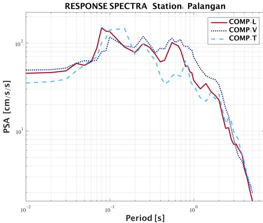
Figure 16. Acceleration response spectra at Palangan station at about 69 km epicentral distance.
