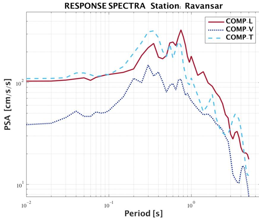
Figure 18. Acceleration response spectra at Ravansar station at about 72 km epicentral distance.
