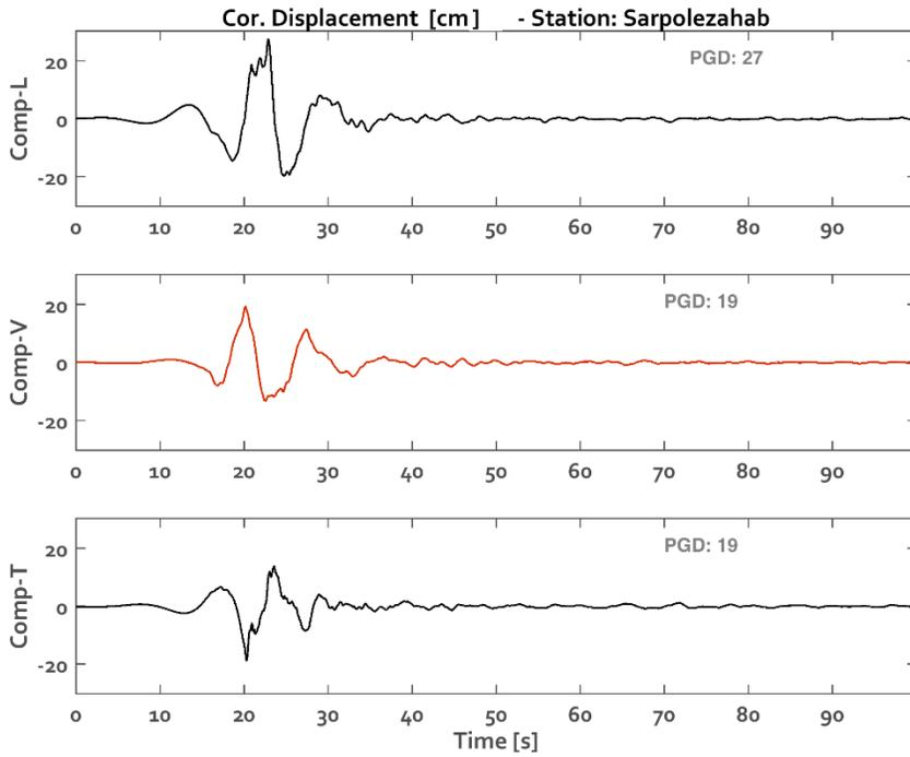
Figure 7. Recorded displacement time history at Sarpol-e Zahab station at about 40 km epicentral distance.
