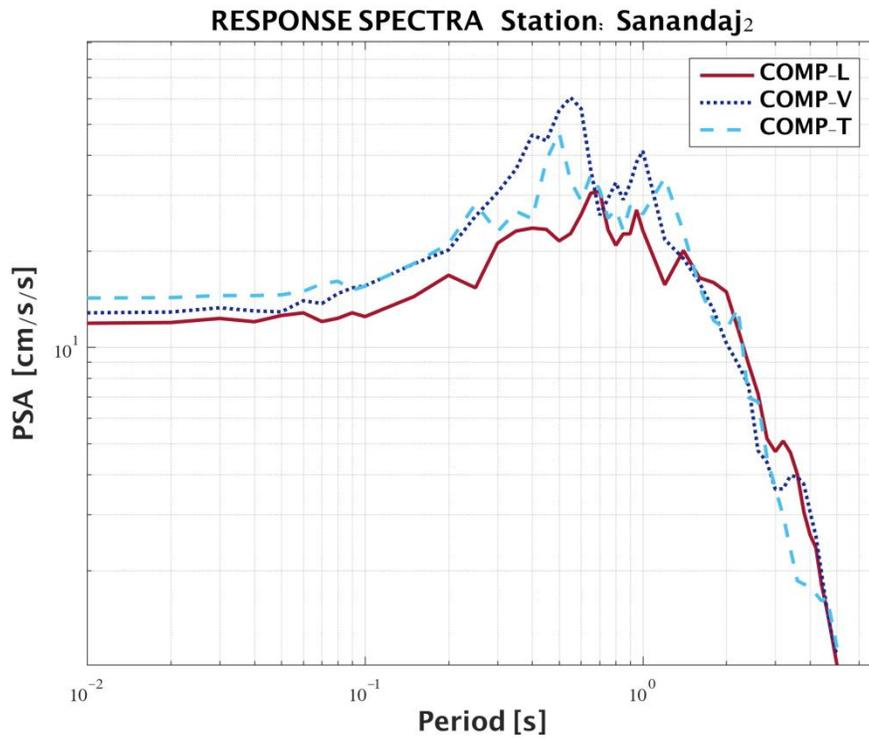
Figure 22. Acceleration response spectra at Sanandaj2 station at about 113 km epicentral distance.
