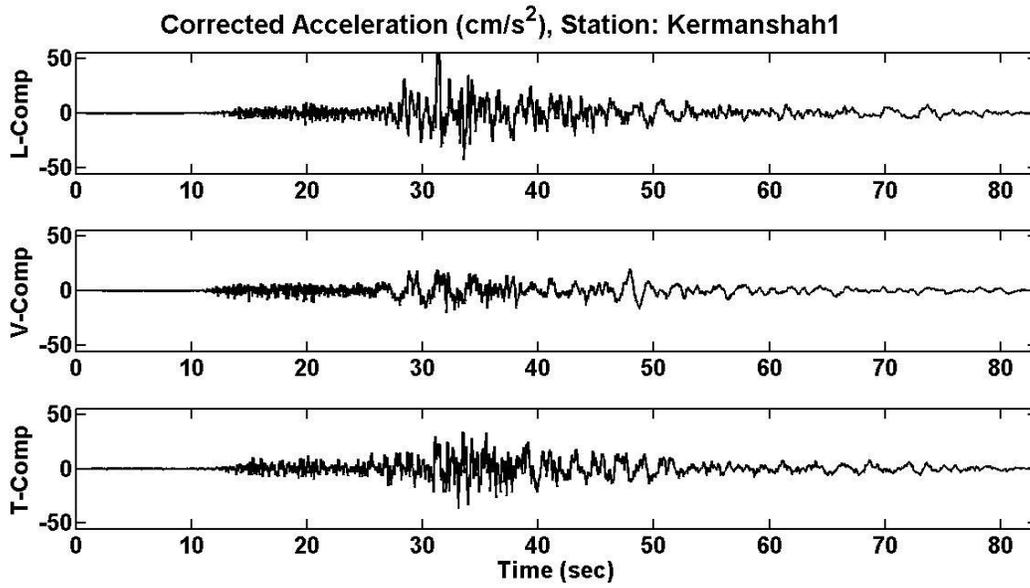
Figure 23. Recorded acceleration time history at Kermanshah1 station at about 122 km epicentral distance.
