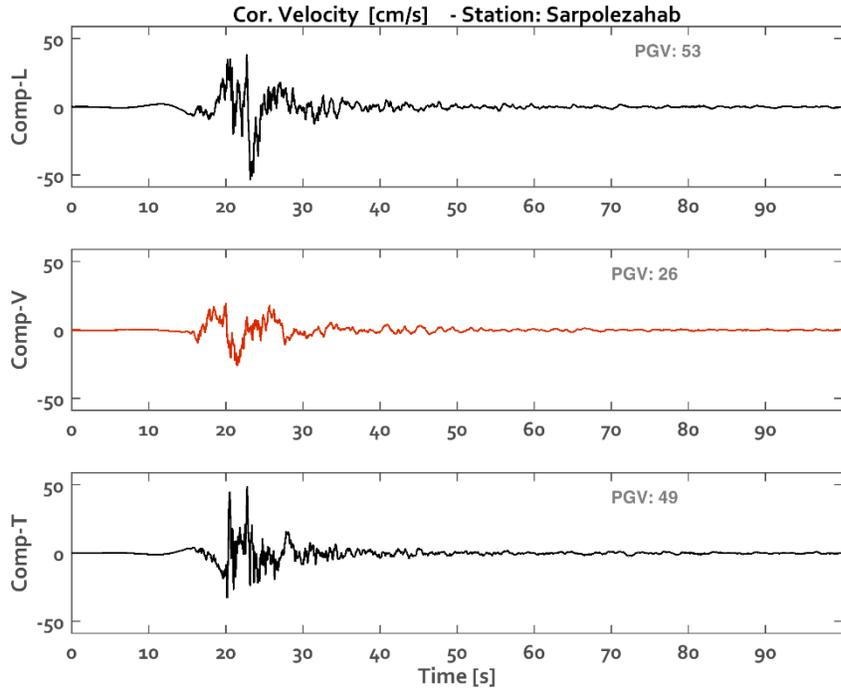
Figure 6. Recorded velocity time history at Sarpol-e Zahab station at about 40 km epicentral distance.
