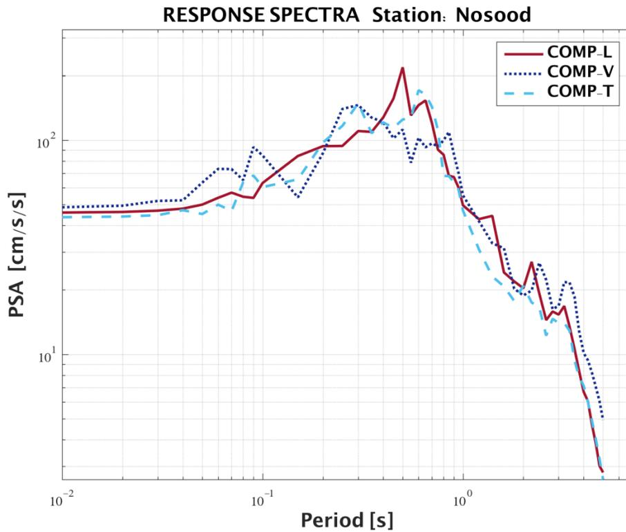
Figure 12. Acceleration response spectra at Nosood station at about 45 km epicentral distance.
