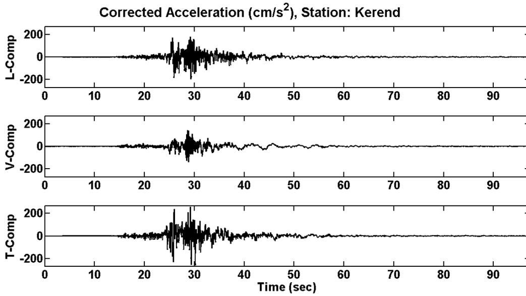
Figure 9. Recorded acceleration time history at Kerend station at about 70 km epicentral distance.
