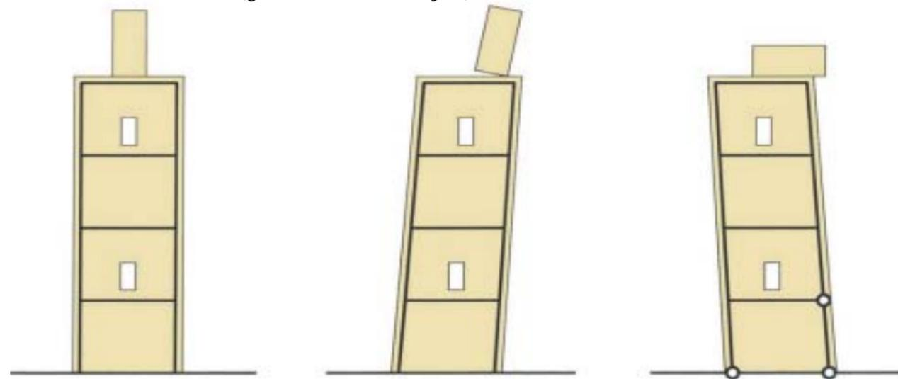
9.6.1 Failure model; In this example incipient plastic hinging is observed in base of tower.
