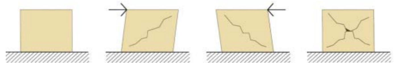
4.5 Reinforced concrete frame – shear damage in non-structural walls.
