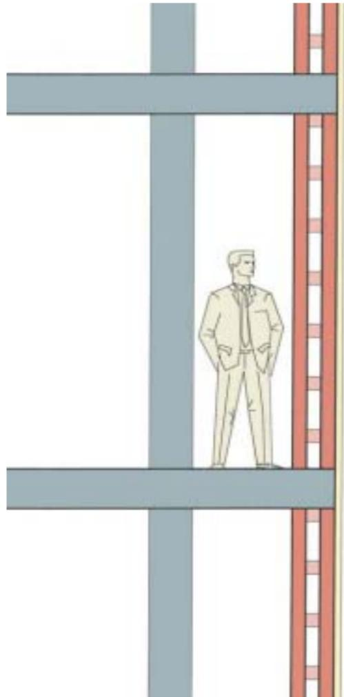
4.2.1 Most RC buildings in Al-Hoceima are clad with a cavity masonry wall system based on two identical skins of hollow brick units tied together with soldier courses laid across the cavity.
