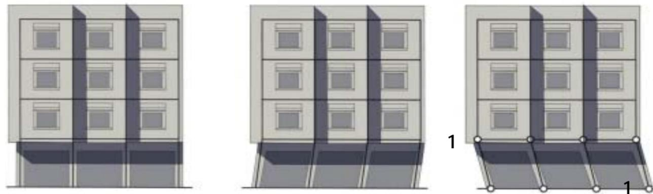
4.9.5 Failure model; Very stiff upper floors drift over an open plan ground floor with insufficient resistance to moments in column to slab connections resulting in plastic hinges (1) and permanent drift.
