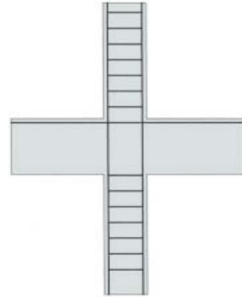
**4.1.1 This is poor practice;** Vintage concrete structures and those which do not incorporate seismic resistant design criteria have poor column to beam and column to slab connections. With emphasis on design for static loads, slabs tend to be very stiff and much more stronger than columns. Columns deform and plastify long before beams or slabs. The majority of buildings analysed in Imzuren were of this kind.
