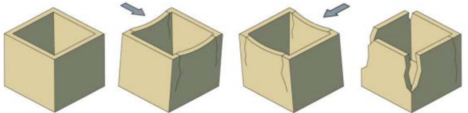
3.5.4 The cyclic reversal of strain in two perpendicular walls meeting at a corner causes brittle failure in unreinforced masonry construction resulting in this widespread earthquake damage.
