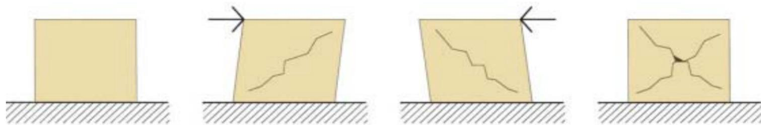
3.4.4 Model of shear damage formation.
