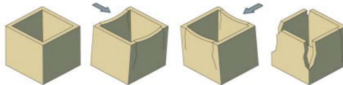
4.4 Reinforced concrete frame – *corner damage to non loadbearing walls*
