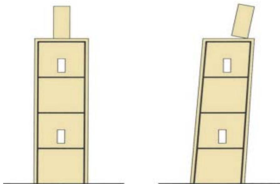
**9.1.1** Scores of mosque minarets were subject to strong shaking in the epicentral area which justifies their inclusion in this report; A simple model for non-structural damage to the mosque lantern is shown above. All mosque minarets are built to similar geometric specifications; a RC frame with no diaphragm action save for the spiral stairs. Lantern is a non-structural element on the roof.
