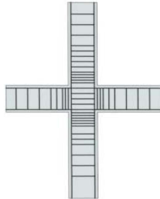
**4.1.2 This is good practice;** In a moment resisting frame, column to slab and beam connections are carefully detailed for rigidity, stiffness and full coupling action between members. A more equal size distribution between vertical and horizontal elements is designed to invoke deflection away from connections. There is no evidence that these conceptual principles were applied in recent RC frames in Al-Hoceima.
