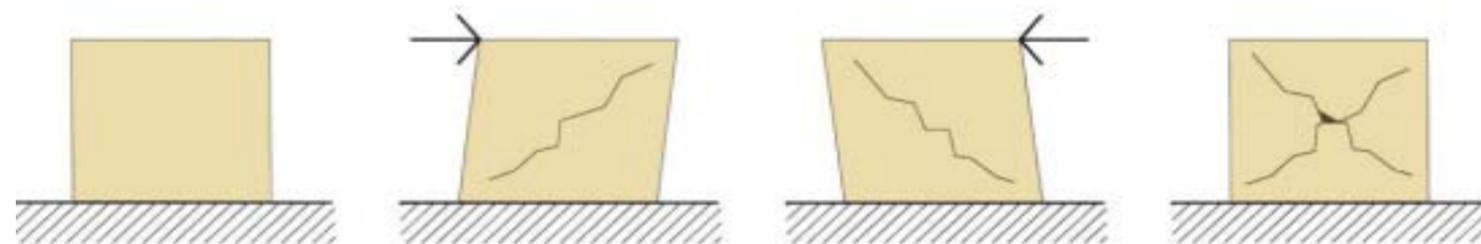
4.6 Reinforced concrete frame – *shear damage in non-structural walls.*
